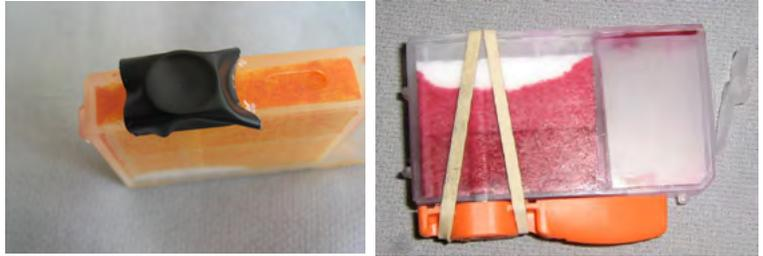
**Step 2.** *Press on the top of the label and feel a depression. Using a pointed knife, remove a small circular part of the label above the ball.*
